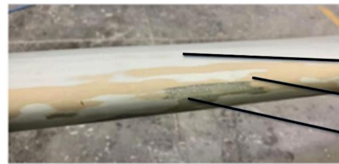
Fæster S, Johansen NF-J, Mishnaevsky L Jr, Kusano Y, Bech JI, Madsen MB. Rain erosion of wind turbine blades and the effect of air bubbles in the coatings. Wind Energy . 2021; 24: 1071–1082. https://doi.org/10.1002/we.2617
